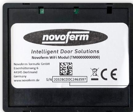
The serial number is located on the back of the WiFi-Module.
