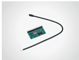
Receiver module with antenna 433 MHz
