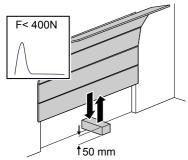
Fig. 7: Checking the force limits
