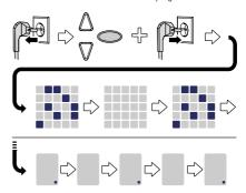
Fig. 6: Deleting all hand-held transmitters programmed for the drive
