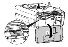
Fig. 10: Opening the drive head cover and determining the radio module type
