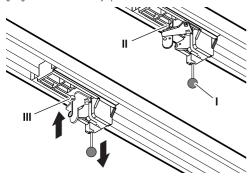
Fig. 9: Disengaging and engaging the drive
