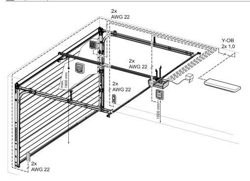
Fig. 3: Example installation of accessories
