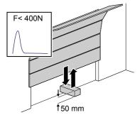
Fig. 7: Checking the force limits
