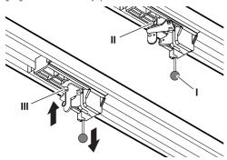
Fig. 9: Disengaging and engaging the drive
